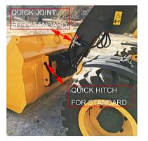
3 Quick hitch for satandard ,can operate a sideshift function or hydraulic
